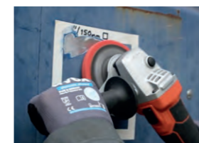
After 2.85 seconds of grinding
