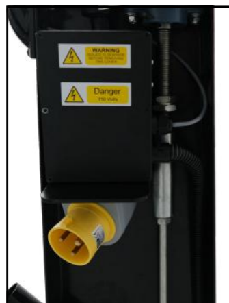
Rear mounted starter box enclosure
