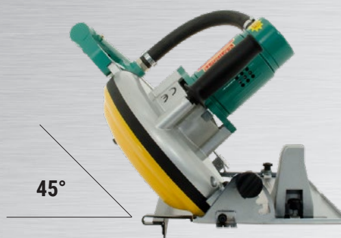
Bevelcut up to 45° (Type 5 115 and 5 1116)
